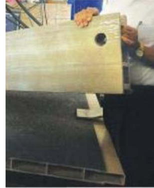
Fig. 3: FRP grate sandwiched between FRP mats
