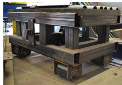
Fig 4: Rolling Load/Moving Cart Platform in WVU-CFC lab
