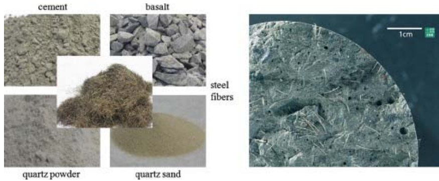
Fig. 2 - 3: Examples of UHPC Components and Embedded Steel Fibers, Source: [14]
