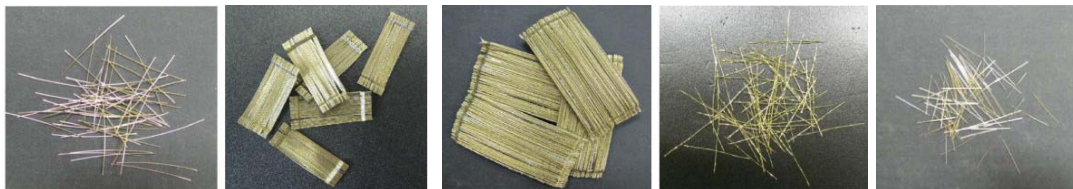
Fig. 12 (a – e): UHPC fiber types: a) Long smooth macro fiber, b) Hooked A macro fiber, c) Hooked B macro fiber, d) Twisted macro fiber, and e) Short smooth micro fiber. Source [16]
