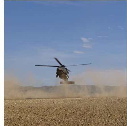
Fig. 3: Brownout conditions from rotor downwash creates a whirlwind of dust and foreign objects.
