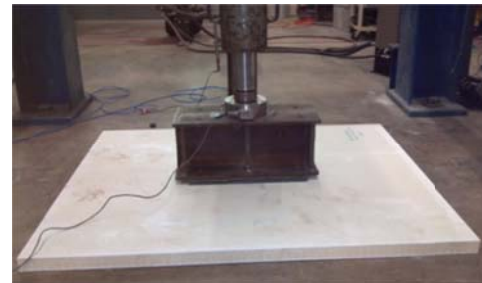
Fig. 1: Single-layer panel used in Alaskan oil fields (under testing at the WVU-CFC lab)
