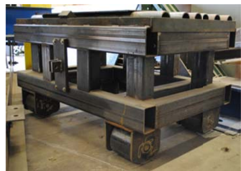
Fig 8: Rolling Load/Moving Cart Platform during testing in the WVU-CFC lab
